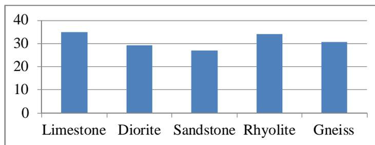
Fig. 8 Mean amplitude values for different species of minerals (dB)
