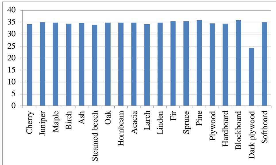
Fig. 5 Mean amplitude values for different species of wood (dB)
